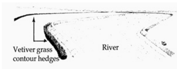
Figure 27. Vetiver protects farmland by stabilizing river banks and by preventing river levees from breaching and flooding into the fields.
